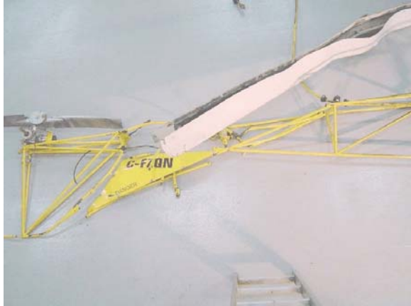
Photo 3. Wreckage reconstruction showing interference of tail boom with rotor
