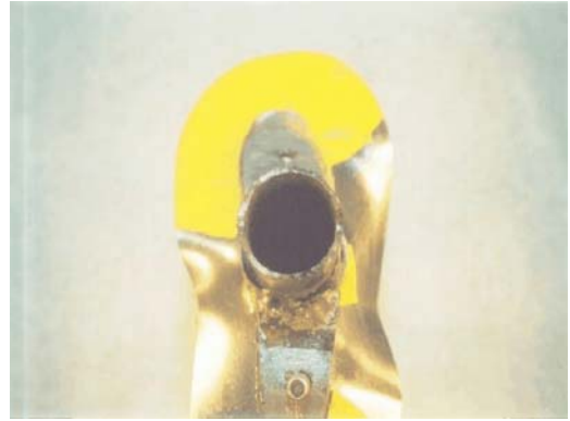
Photo 2. Horizontal stabilizer spar fracture
