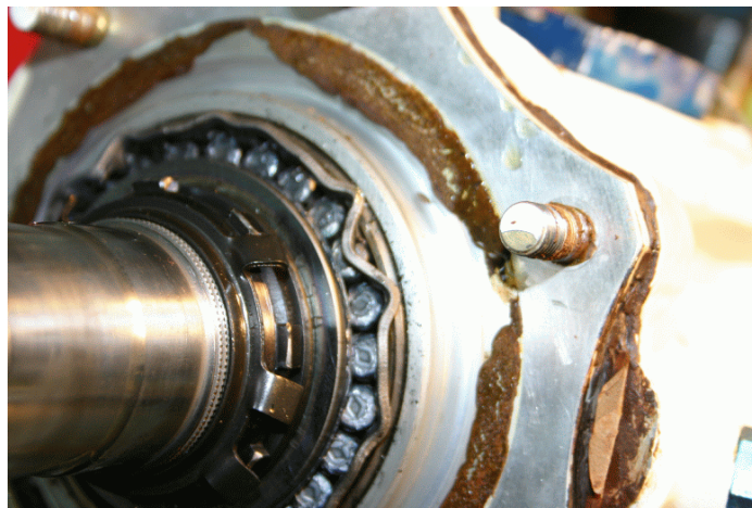
Photo 1. Distorted bearing cage
