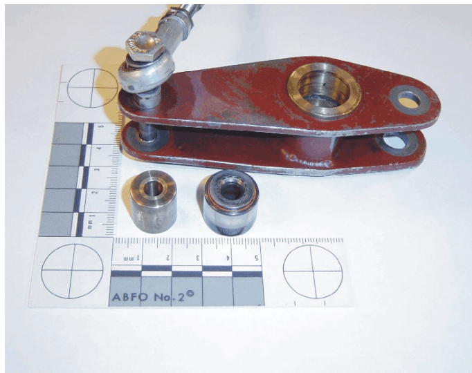
Photo 1. Bellcrank assembly with a part number 5453032-1 roller on the left and a YCRS-12 bearing on the right
