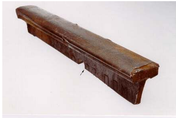
Photo 2. Splice bar bolt hole and web fracture
