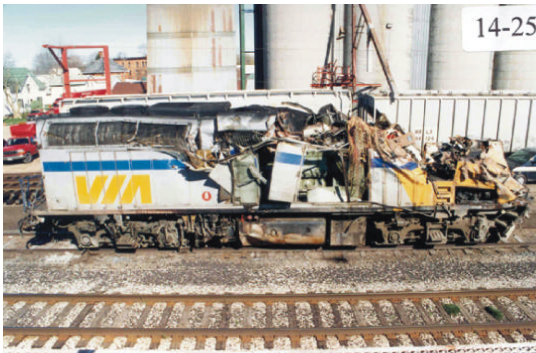
Figure 4 - Right side shown after locomotive was righted. Damage is more extensive at the front right and along the right side of the locomotive.
