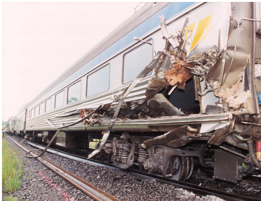
Figure 3—Outside damage from corner of tractor-trailer after rotation
