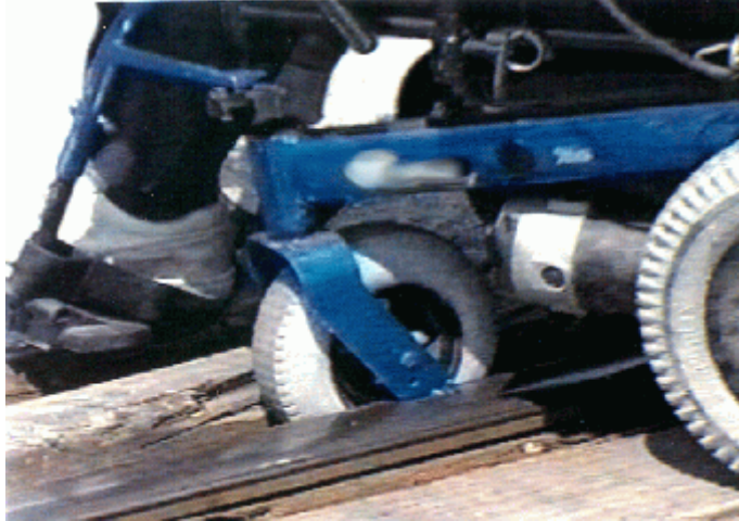
Figure 3 - Wheelchair of the same type as one of those involved in the accident, but not with identical specifications, with a castor wheel in the field side of the rail.
