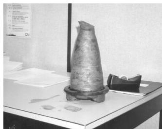
Figure 9 - View of end cap and remaining portion of axle stub
