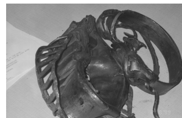
Figure 10 - Pieces of internal roller bearing parts
