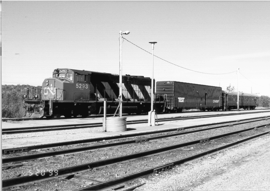
Figure 20 - Typical CN TEST train configuration showing a freight locomotive, a highly instrumented box car and a dedicated track geometry car
