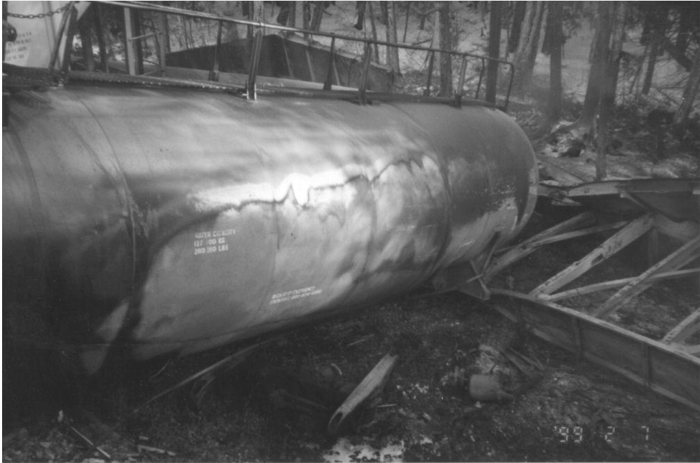
Figure 3 - Fire-damaged jacket of loaded tank car of LPG (CGTX 63501)
