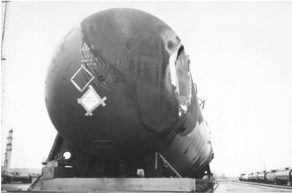
Figure 4 - Damaged benzene tank car (AGEX 1001)
