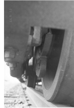
Figure 17 - End view of roller bearing housing on railiner
