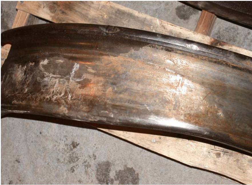
Photo 3. Plastic deformation of the running surface on wheel L2
