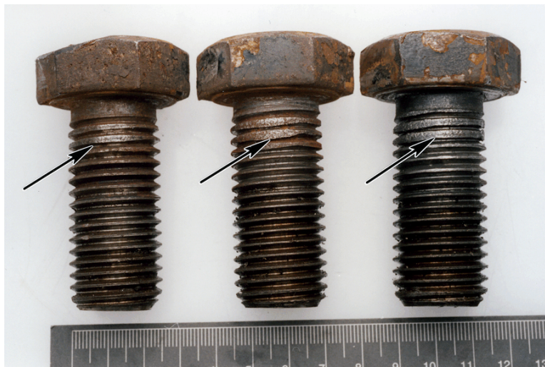
Photo 4. Fretting wear on threads of cap screws
