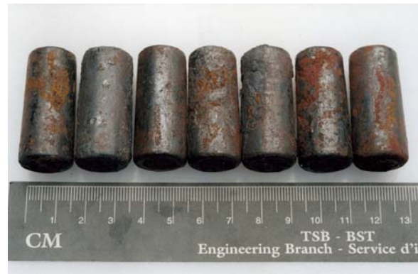
Photo 3. Inner rollers from R-2 bearing
