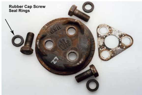
Photo 2. Rubber cap screw seal rings, with cap screws, end cap, and locking plate, in roller bearing at L-2 and R-2 positions
