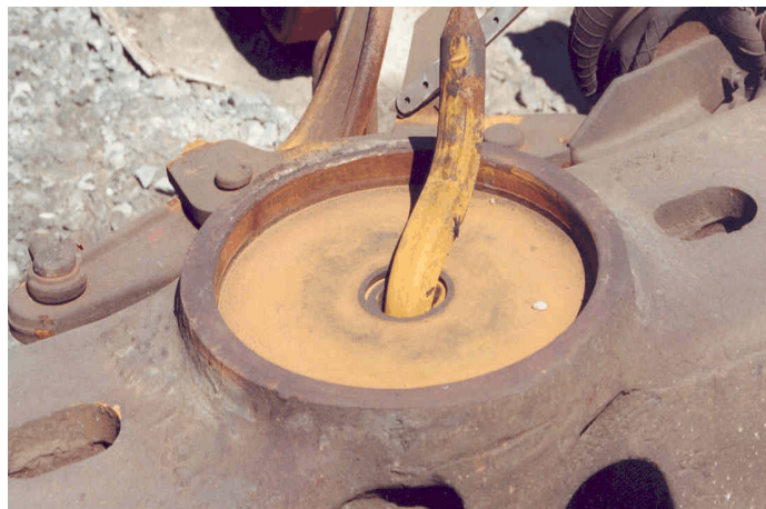
Figure 4. Centre plate and pin of truck D
