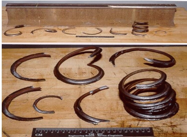
Figure 1. Curled strips of flow lip sheared from the rail
