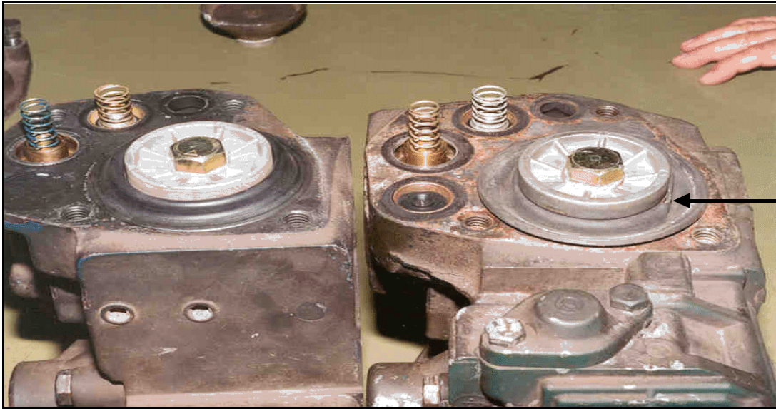
Figure 2 Normal diaphragm (left) compared to defective diaphragm (right).
