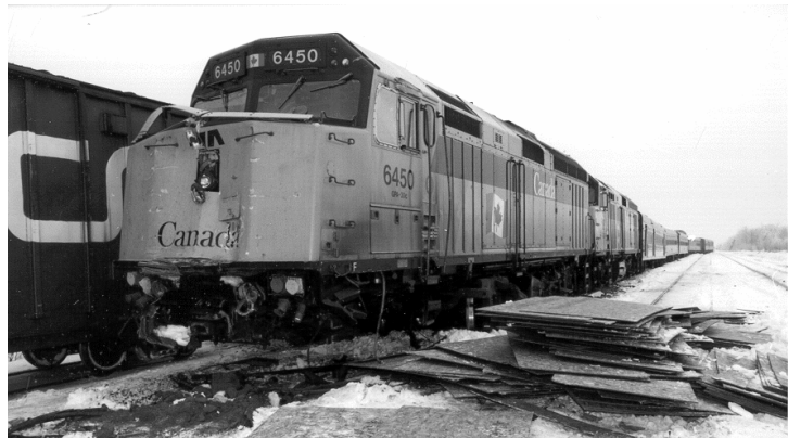
Photo 2. Some of the damage to lead locomotive VIA 6450. Note displaced front truck under centre of locomotive (which damaged the battery boxes and diesel fuel tank) and impact marks on collision posts on the front of the locomotive.
