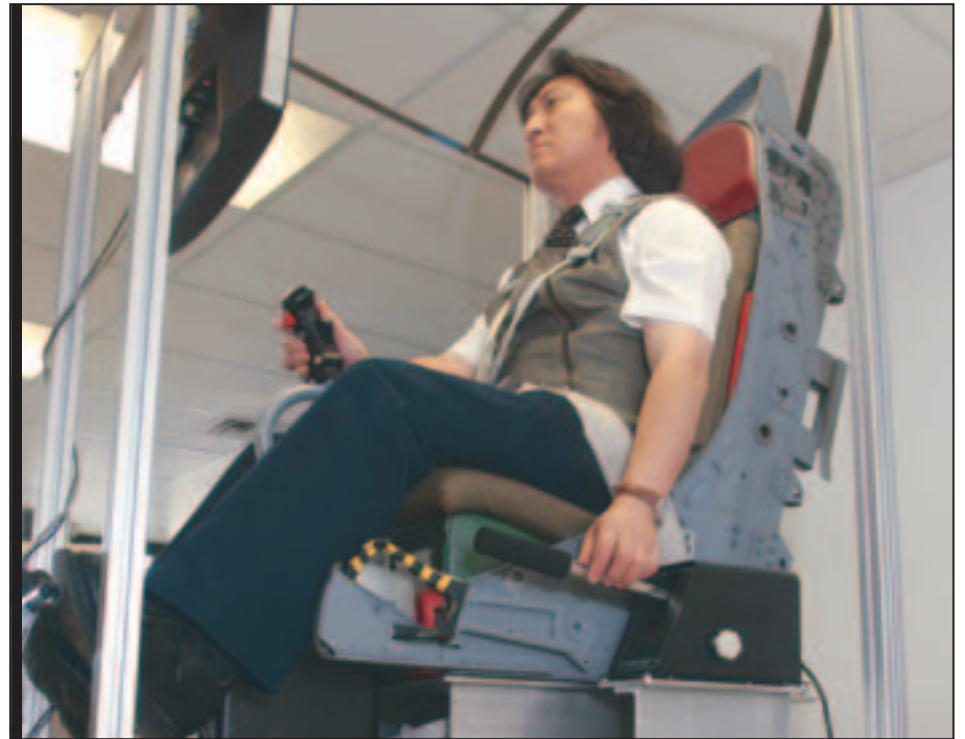
Dr. Bob Cheung of DRDC-Toronto sits in a simulated helicopter cockpit wearing a prototype of the buzzing garment he is developing for aircrew.
