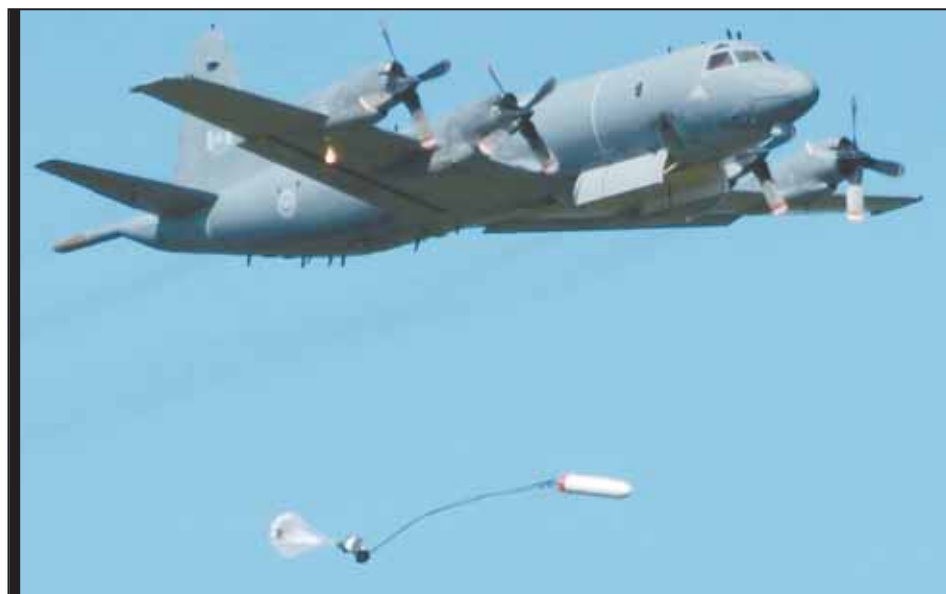
A CP-140 Aurora drops a survival kit air droppable, the first operational drop of its kind in the aircraft's 27-year history.
