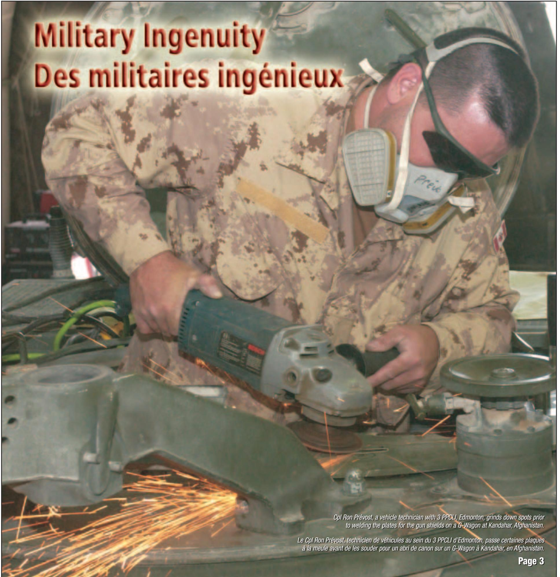
*Cpl Ron Prévost, a vehicle technician with 3 PPCLI, Edmonton, grinds down spots prior to welding the plates for the gun shields on a G-Wagon at Kandahar, Afghanistan.*
