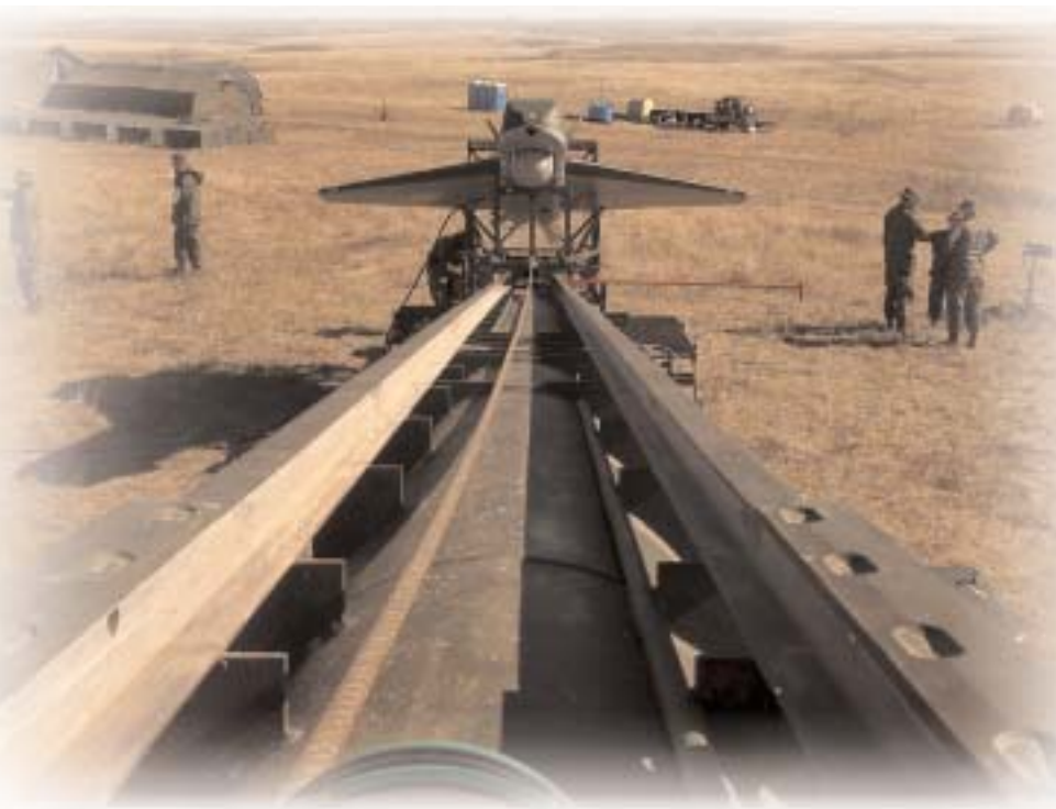
An Aerial vehicle sits on the launcher as launch preparations take place. Those preparations can take up to two hours.
