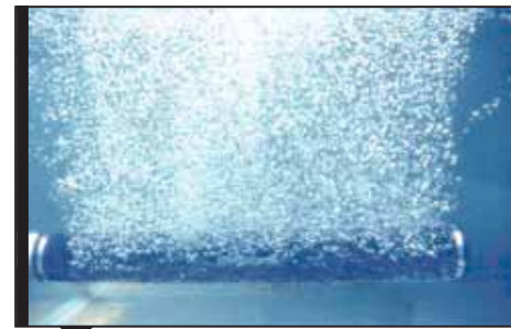
The Bubble curtain at work. Here, you can see the "bubble system" as it appears underwater.
