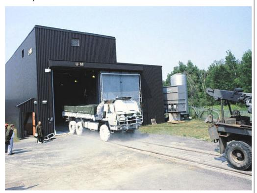
This large climatic chamber with railway access accommodates the largest and heaviest single-unit railway vehicles, highway or off-road transport vehicles, prototypes and commercial products.
