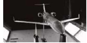
A three-point mount is commonly used for static tests, while sting mounts are used for unsteady measurements with oscillating models
