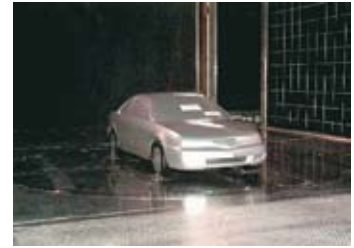
Typical installation for surface vehicle aerodynamics experiments (photo courtesy Honda R&D Americas)
