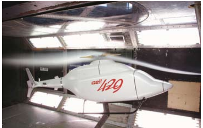
Model of prototype helicopter undergoing tests
