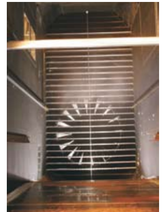
PIWT test section with spray bars in operation
