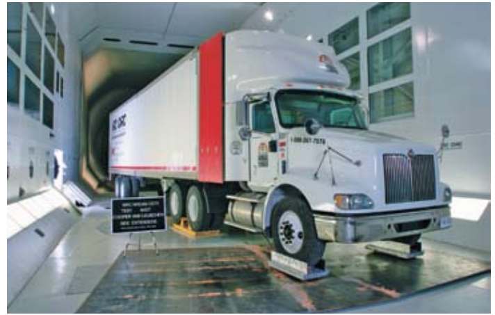
Aerodynamic test on a full-scale truck
