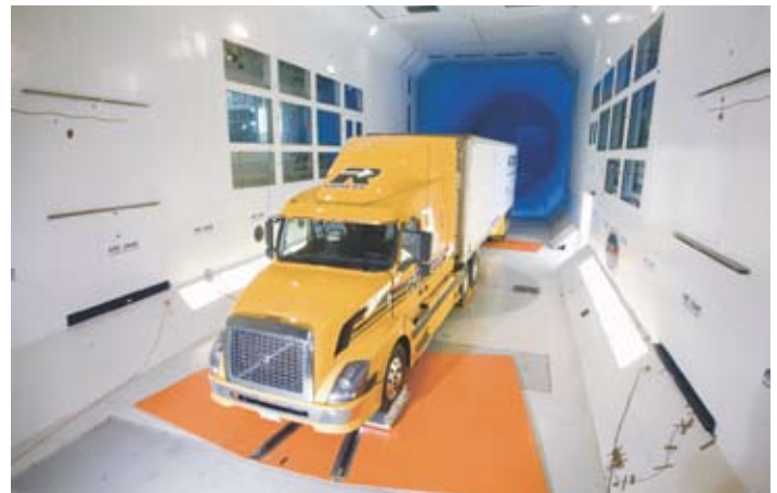
Full-scale tractor-trailer in the NRC 9 m x 9 m wind tunnel (speed: 200 km/h). Trailer was cut in two to bring it into the tunnel
