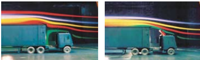
Multiple smoke streams show how a cab-mounted deflector protects the trailer and saves 13,000 litres per year at 105 km/h
