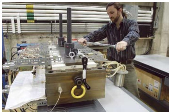
Modular mould used to fabricate composite parts
