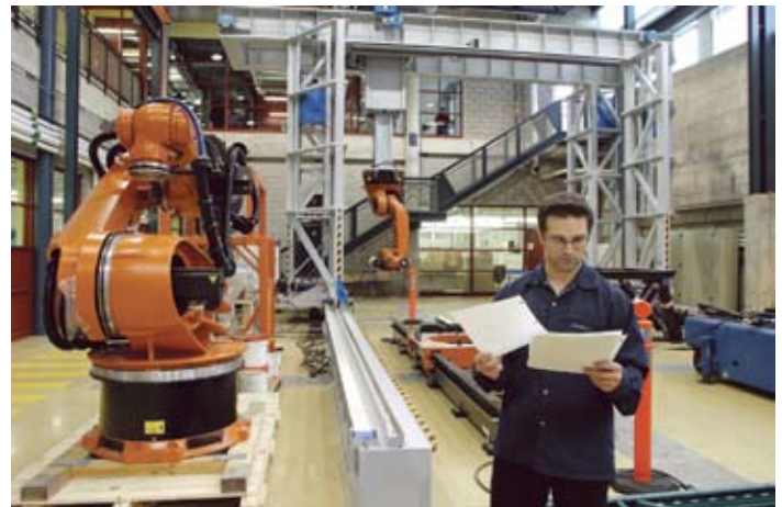
Gantry system with industrial robots
