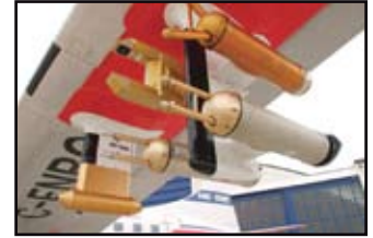
Cloud physics probes mounted on wing pylons
