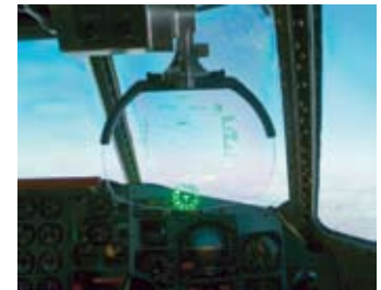
Heads Up Display installed on the NRC Falcon 20
