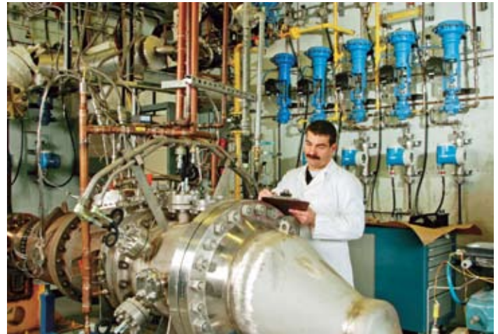
High-pressure (300 psig) test rig
