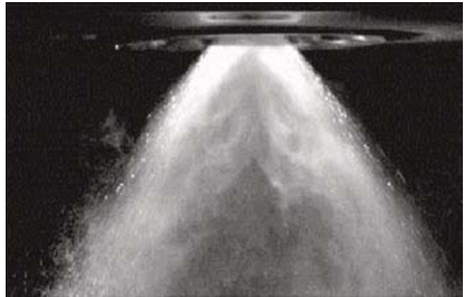
Flow visualization using laser sheet illumination from an industrial nozzle
