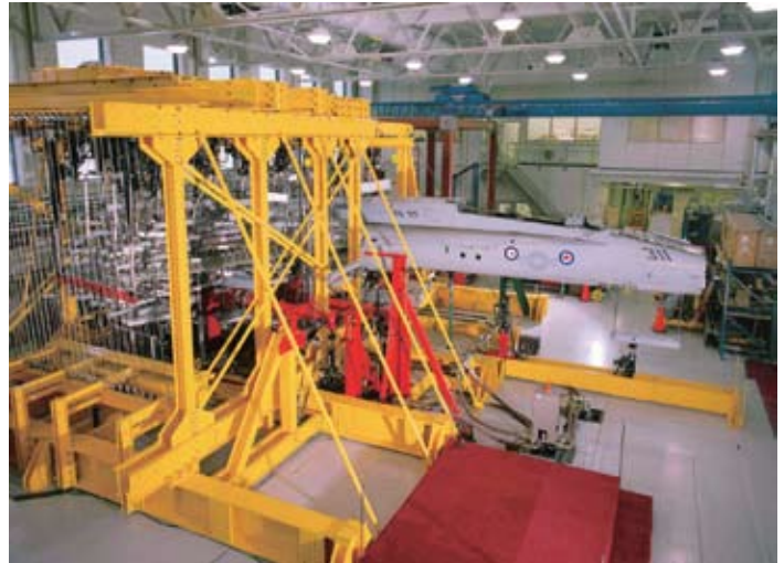
Full-scale fatigue tests on CF-18 wing for International Follow-On Structural Test Program
