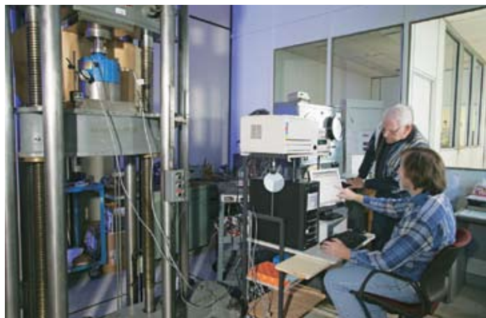
Calibrating the 100,000 lbf load cell
