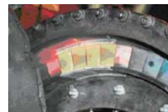
Thermal barrier coated components, internally cooled
