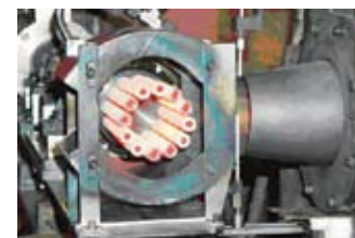
Hollow specimens, internally cooled
