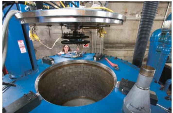
Lowering a turbine disk into the spin rig
