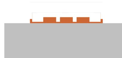
Template is released and a polymer mask remains on the substrate
