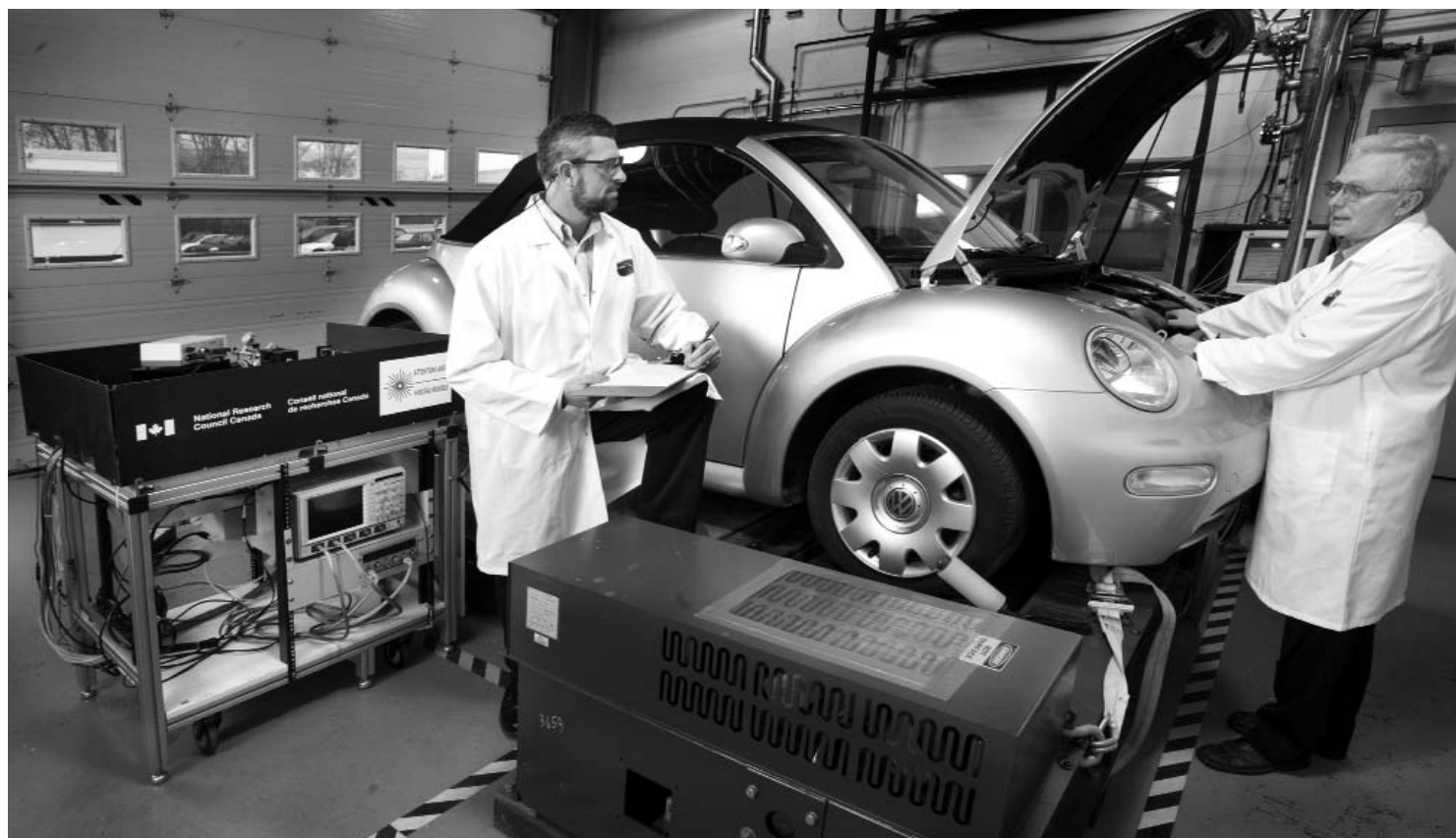
NRC's Greg Smallwood and Reg Smith use an NRC-patented technology to measure particulates in vehicle emissions – in the lab and on the road.
