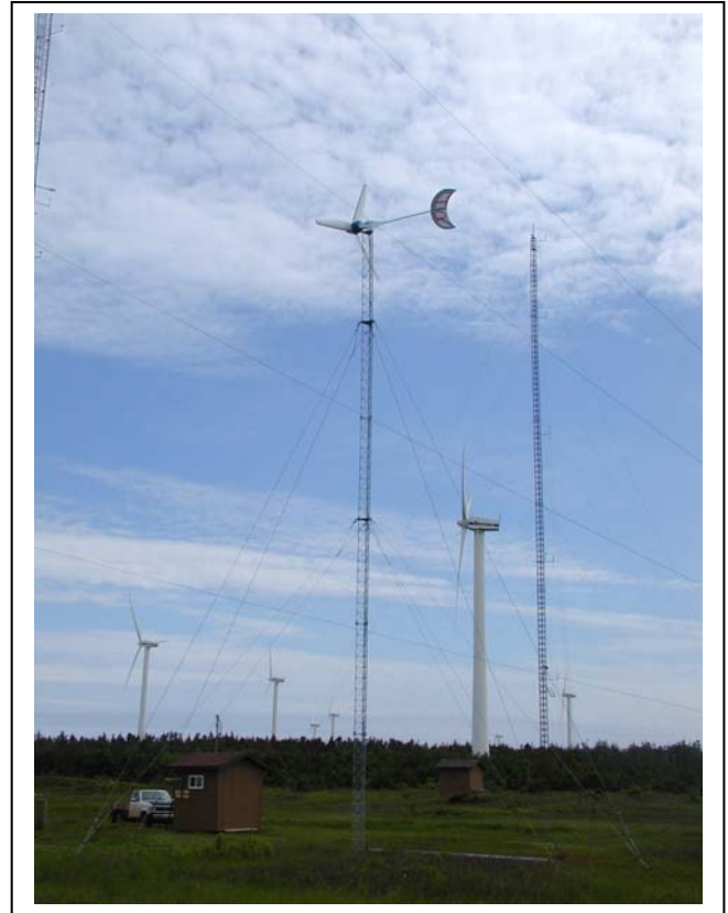
2.5 kW Small Wind Turbine in Testing and Large Turbines Producing Electricity at the Wind Energy Institute of Canada – Source: WEICan
