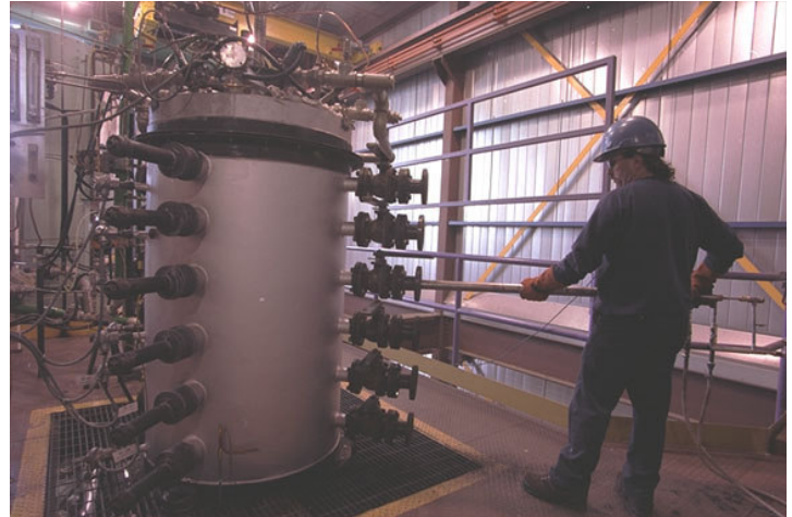
CEPG staff performing temperature measurements on the vertical combustor
