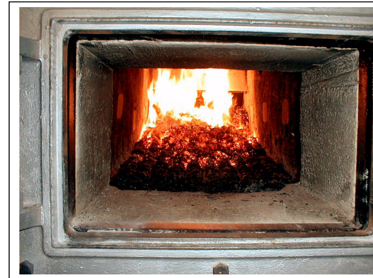
Biomass combustion in a moving grate furnace
