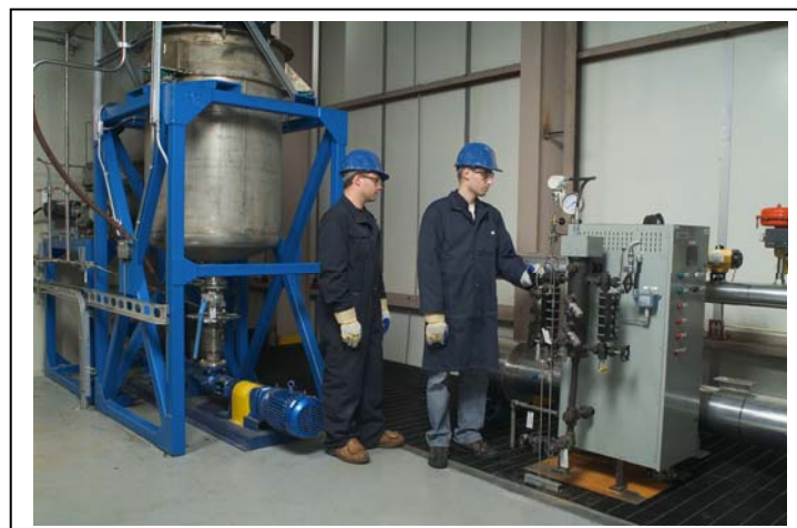
Image below: The gasifier is capable of running with a dry feed or a slurry feed.
