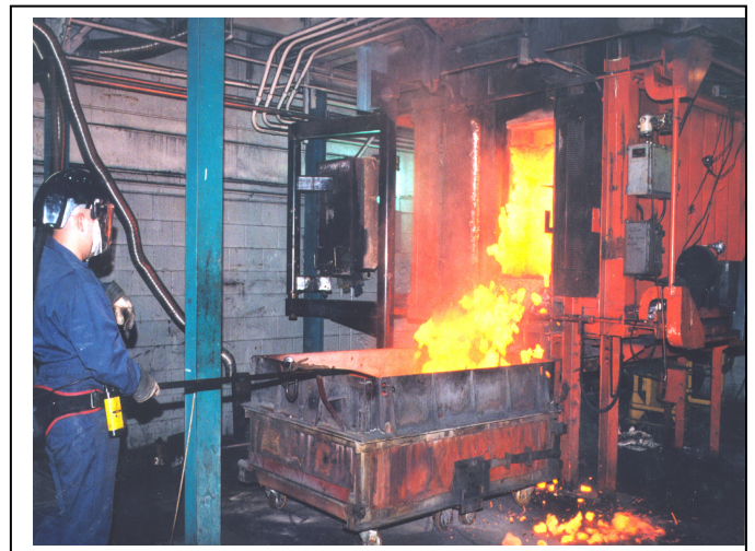
Discharging of metallurgical coke from CETC-Ottawa moveable-wall pilot oven
