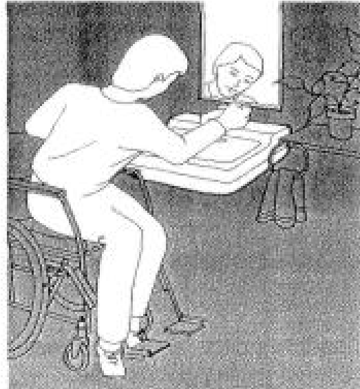
Side access to a standard basin. Notice the mirror can be tilted to different angles.
