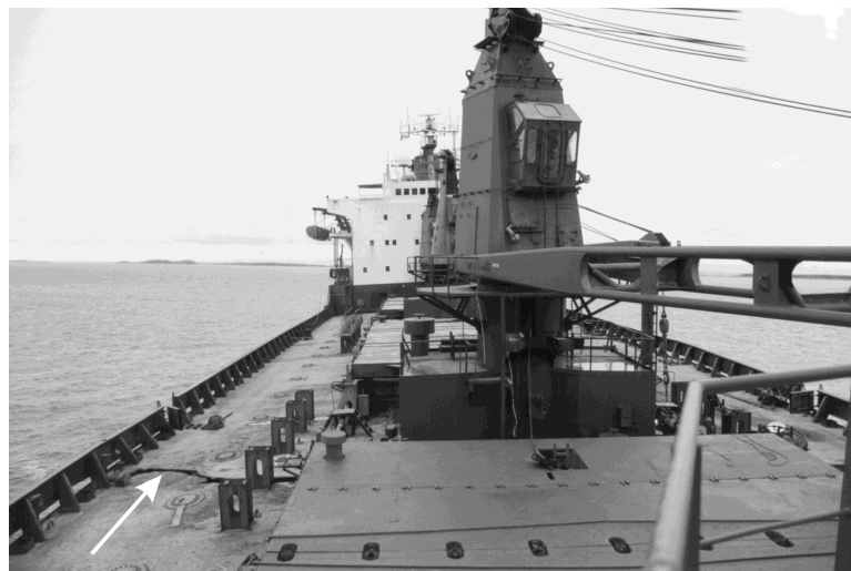
Photo 4. Main deck fracture (at arrow)
