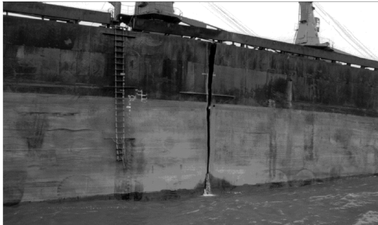
Photo 2. Starboard side fracture
