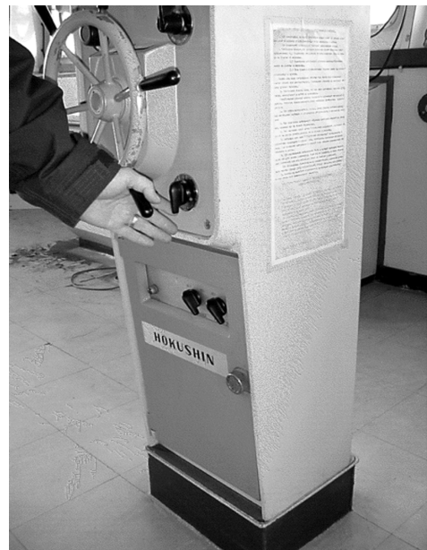
Photo 1. Simulation of accidental switch activation
