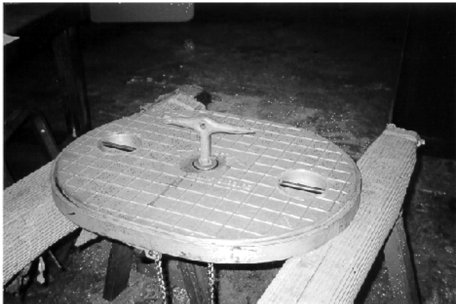
New aluminum flush-deck cover designed by Manly Marine Closures, Ltd., identical to that which became dislodged during the occurrence. Note the recessed locking bolt, with its fitted bronze key in place.
