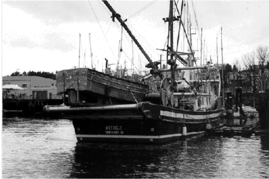
The "WESTISLE" on 3 March 1999, secured at the premises of Alberni Engineering in Port Alberni, B.C. Note the stern of the work boat is located to port of the centreline, where it was placed at the time of the occurrence.
