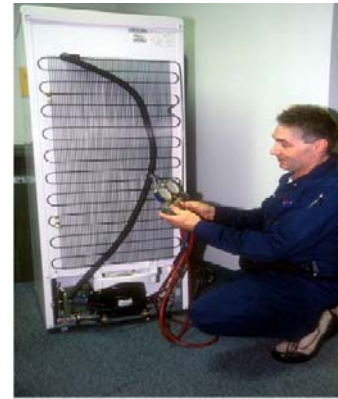
Freon is safely removed from all old fridges before shipping.
