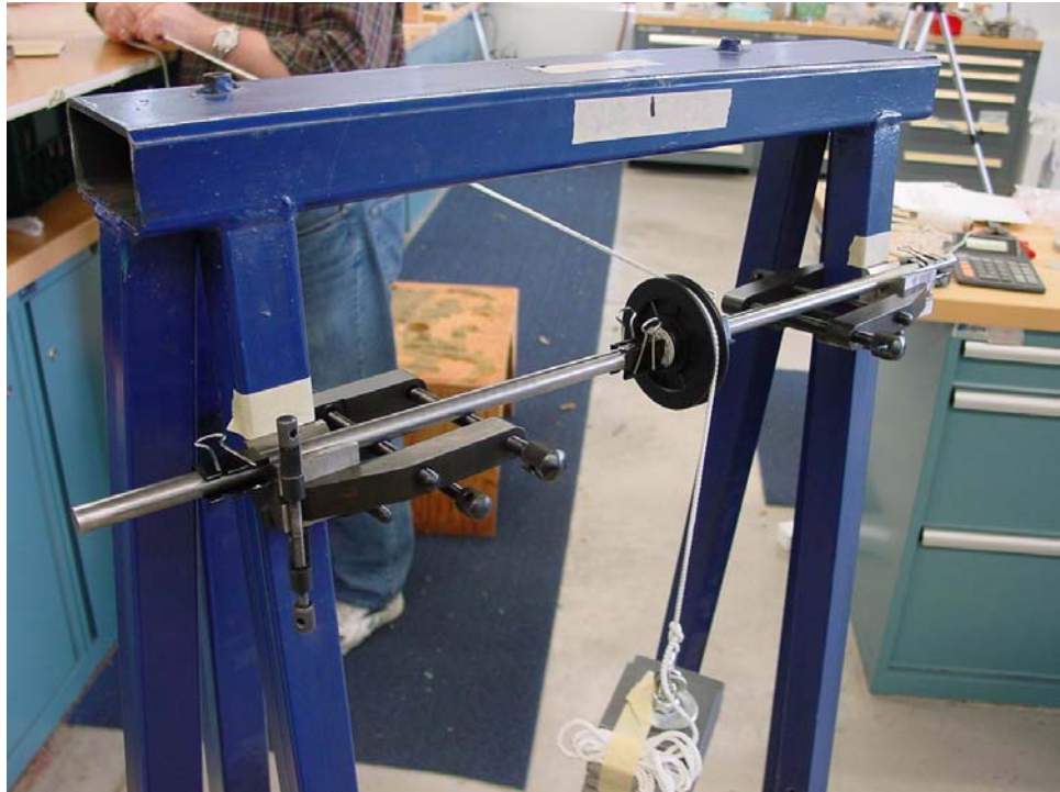
Figure 15: Pulley set up for angled tests
