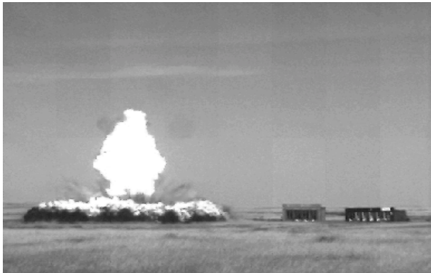
Test for blast resistance of windows mounted in structures at right.
