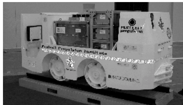
Canadian-built mine locomotive – the world’s first fuel cell industrial vehicle.
