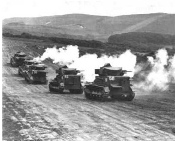
Light Tank Mark III: The majority of British tanks at the start of the Second World War were light machines, too lightly armoured to apply the theories of the armoured warfare enthusiasts. (Photo courtesy of the author)
