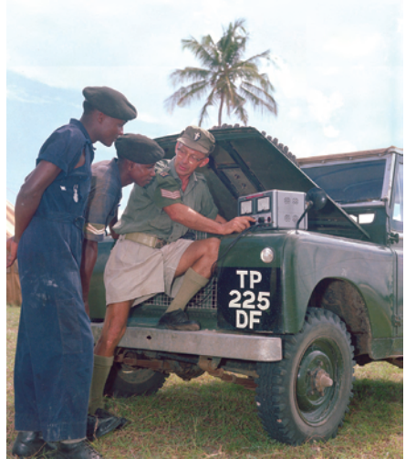
Sgt John Rogers, RCEME, teaches how to use a generator tester
