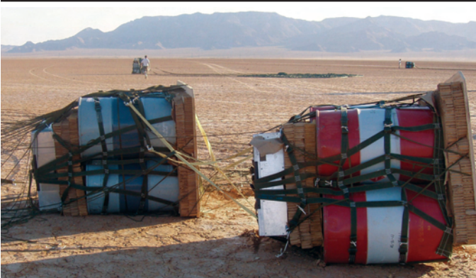
Four AGAS land on target after having been dropped from 13 000 ft with the use of in-service round cargo parachutes
