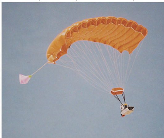
MMIST's PGADS system, the SHERPA flies under its ram-air canopy during a test flight
