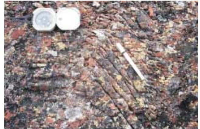
Figure 8. The dominant approximately 100^\circ fracture set shows dextral rotation to about 340^\circ by two kink bands that trend about 040^\circ . These kinks are linked by a set of fractures trending about 340^\circ . The compass is oriented at 098^\circ and the pen 040^\circ . The approximately 100^\circ set of fractures are parallel to a regional set of normal faults trending about 100^\circ . The approximately 340^\circ set of fractures are parallel to a regional set of approximately 340^\circ strike-slip faults of dextral displacement.
