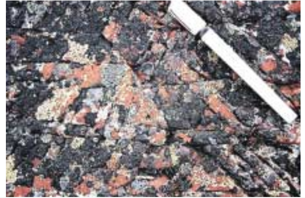
Figure 10. Three fracture sets, trending about 100^\circ , 040^\circ , and 40^\circ , are developed. The pen is oriented at 340^\circ . The approximately 100^\circ fracture set crosscuts the other fracture sets in the left-central part of the photograph.
