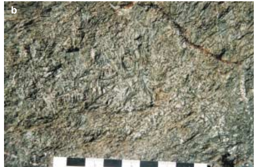
Figure 3. Spinifex-textured ultramafic rocks of the Red Lake belt. a) bladed olivine komatiite, Balmer assemblage, Golden Arm; b) acicular clinopyroxene komatiitic basalt, Ball assemblage, Miles Creek.
